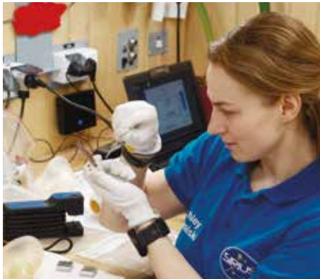
Ashley replaces the flasks in the device that measures gas composition of the lungs
