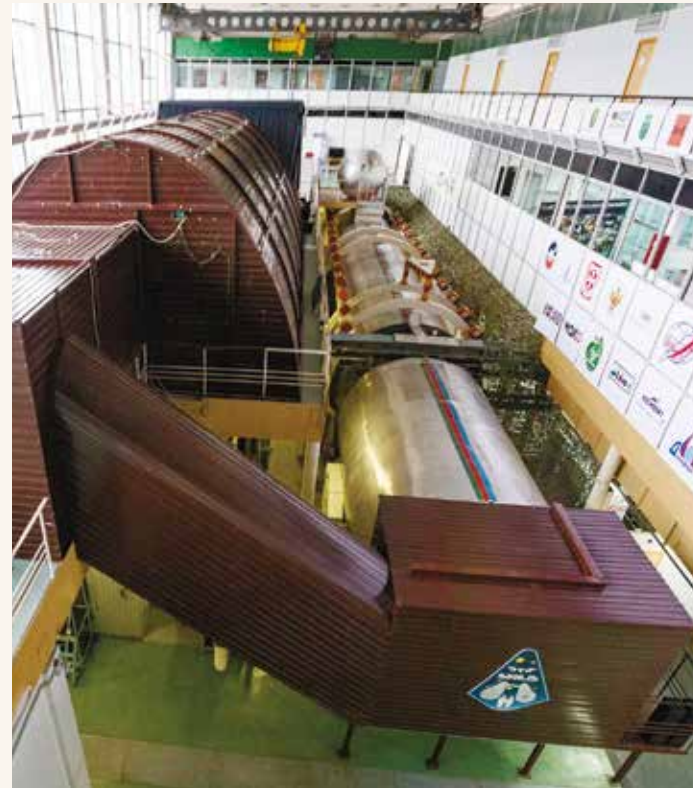
The IBMP RAS ground test facility where the SIRIUS-21 isolation experiment took place. The space volumes and ergonomics of the five modules are as close as possible to space station conditions
