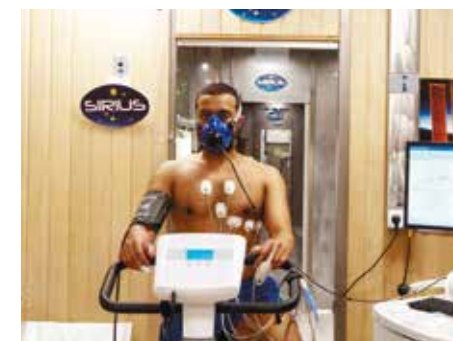
Saleh is wearing a blood pressure cuff, ECG sensors, a pulse oximeter and a mask that records the composition of exhaled air
